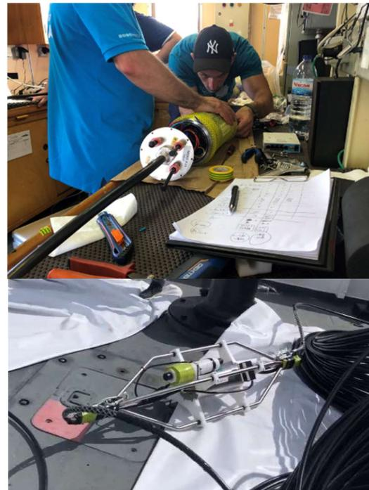
Figure 5: INESC TEC researchers mounting a N<sup>2</sup>ODE on the cable (top) and a N<sup>2</sup>ODE mounted on the mechanical structure, ready for deployment (bottom)
