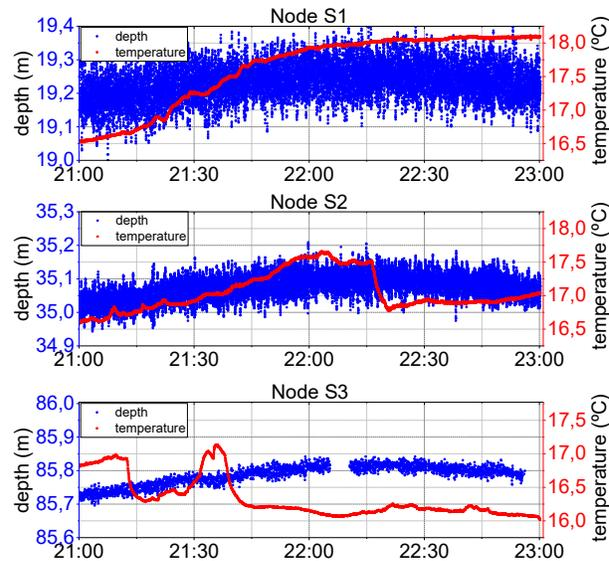
Figure 10. Measurements of water temperature and water depth of nodes 1, 2 and 3 on the 10<sup>th</sup> of September 2023.
