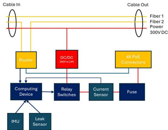
Figure 3: final architecture of the N<sup>2</sup>ODEs
