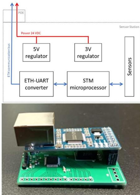
Figure 7. The top image shows the electric scheme of the Sensor station and the bottom image a photograph of the printed circuit board.
