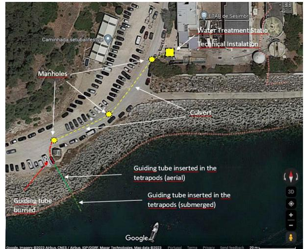
Figure 2: Map showing the components of the shore station and the landing of the cable.
