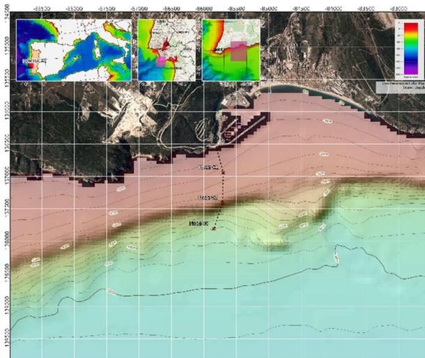
Figure 1: Chart showing the final layout and location of the cabled system and nodes deployed ashore Sesimbra, in Portugal.
