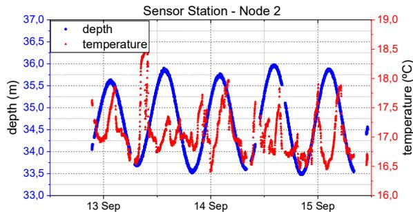
Figure 11. Measurements of water temperature and water depth of node 2 from the 12<sup>th</sup> to the 15<sup>th</sup> of September 2023.
