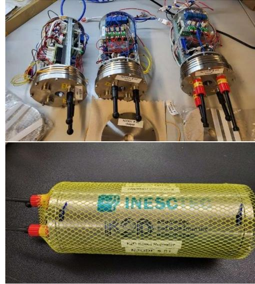
Figure 4: Three N<sup>2</sup>ODEs with exposed electronics (top) and a closed N<sup>2</sup>ODE (without cable penetrator) (bottom)
