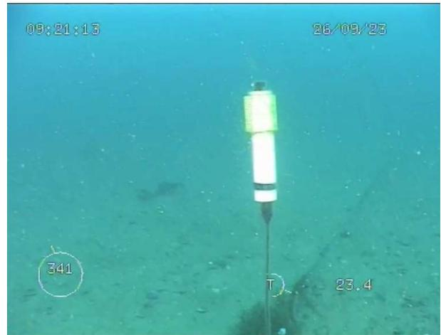
Figure 8. The top image shows node 1 together with the spiral source satellite, which also comprises a hydrophone; The bottom image shows the TP-1 hydrophone placed in nodes 2 and 3.
