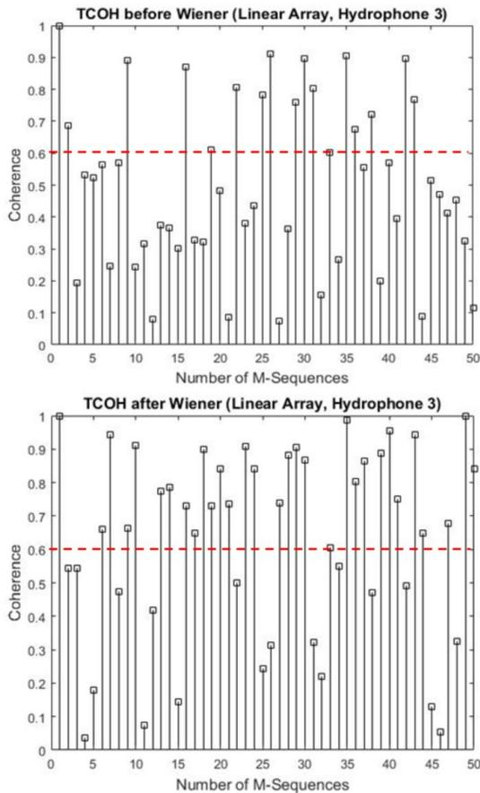
Fig. 4. Temporal coherence before (top plot) and after Wiener filter (bottom plot) of bitstreams recorded by hydrophone #3 of the vertical linear array. Dashed line in red, at 0.6, marks the threshold for TCOH
