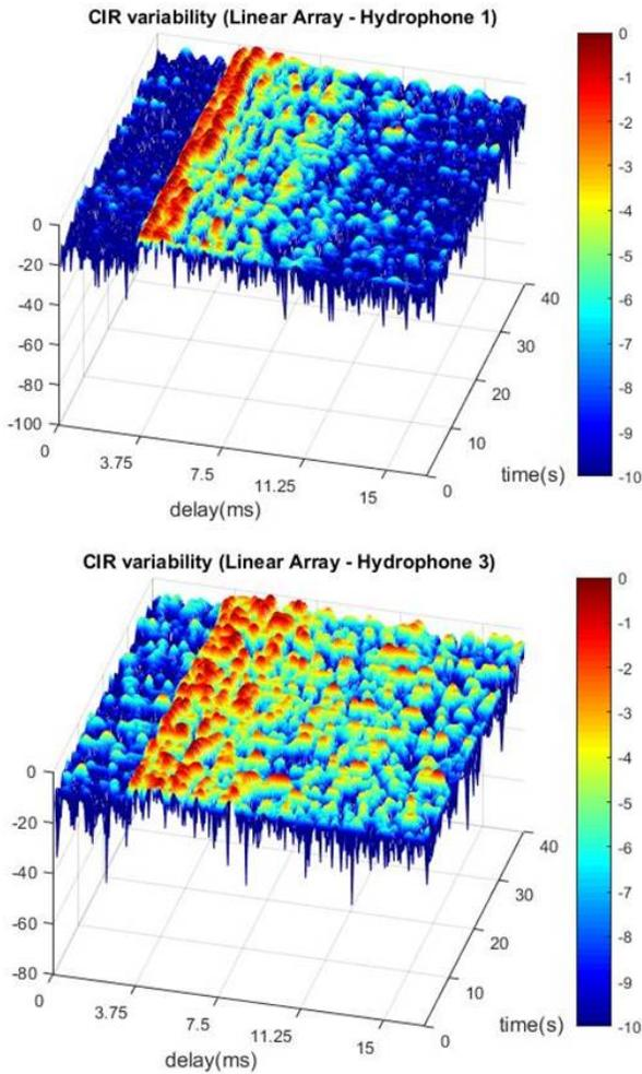
Fig. 1. CIR variability in time, estimated using 50 bitstreams ( $F_c$ :7.5 kHz,  $BW$ : 3 kHz). Data were recorded by hydrophone #1 (top plot) and #3 (bottom plot) of the vertical linear array, installed at 1.5 m and 4.5 m above the bottom in approximately 8 m water depth.
