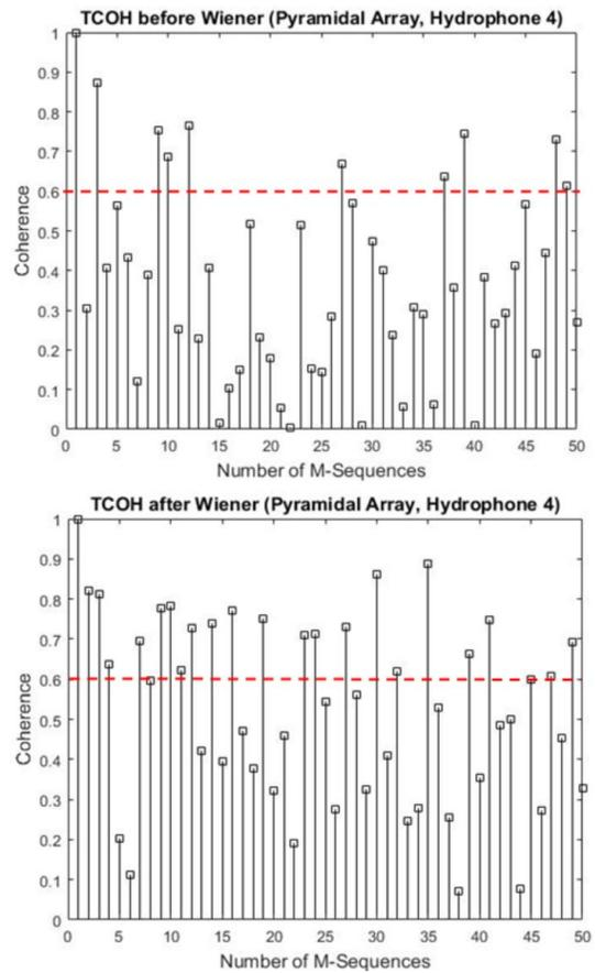
Fig. 5. Temporal coherence before (top plot) and after Wiener filter (bottom plot) of bitstreams recorded by hydrophone #4 from pyramidal array. Dashed line in red, at 0.6, marks the threshold for TCOH
