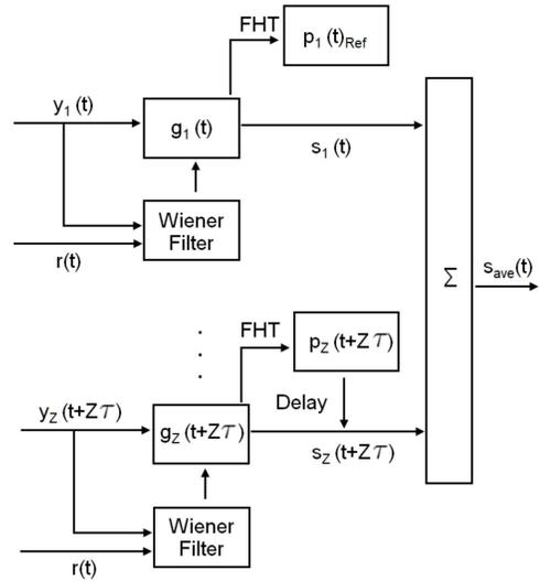
Fig. 3. Diagram of Wiener filtering, CIR estimation using Hadamard transform and coherent averaging of sequences whose TCOH was above the 0.6 threshold.
