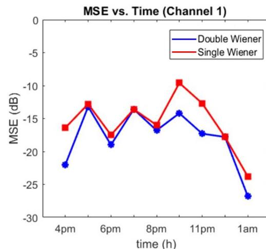
Figure 5: MSE vs. time estimated for channel #1 during the upwelling window, to compare the performance of the single and double Wiener filter.
