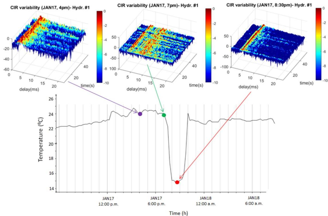
**Figure 3: Top plot: CIR variability in a restricted upwelling time frame from Jan. 17, 4 p.m. to Jan. 17, 8:30 p.m. Bottom plot: temperature evolution in time, measured by a thermistor located close to hydrophone #1, approximately 1.5m above the bottom.**
