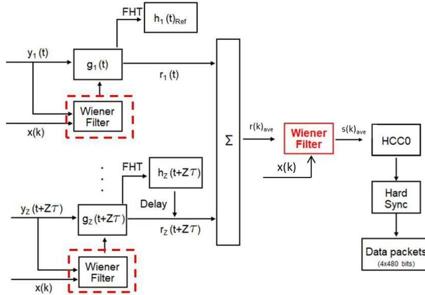
*Figure 2: Diagram of the double Wiener filter communication system shows the following steps: channel equalization (single Wiener filter), soft synchronization, temporal coherent averaging of  $Z$  received bitstreams, the double Wiener filter over the averaged bitstream, probe interference removal (HCC0), hard synchronization, and data retrieval.*
