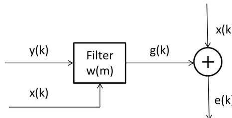
**Figure 1: Diagram of the Wiener filter for linear MMSE estimation.**
