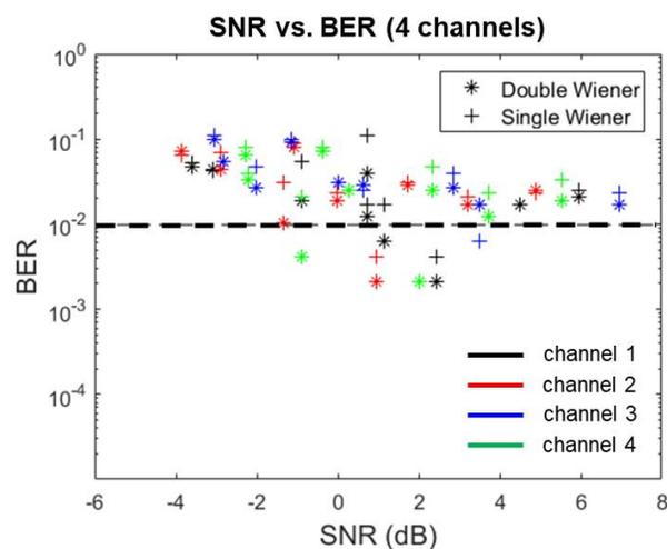
Figure 4: SNR vs. BER estimated for the four channels, independently, using both single and double Wiener filter approaches.
