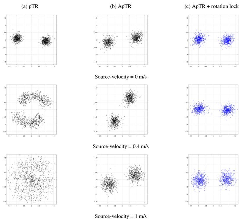
Figure 4: Constellations for moving source and wind-driven modelled surface. Column (a): pTR; Column (b): ApTR without constellation angle correction. Column (c): ApTR with constellation angle correction.
