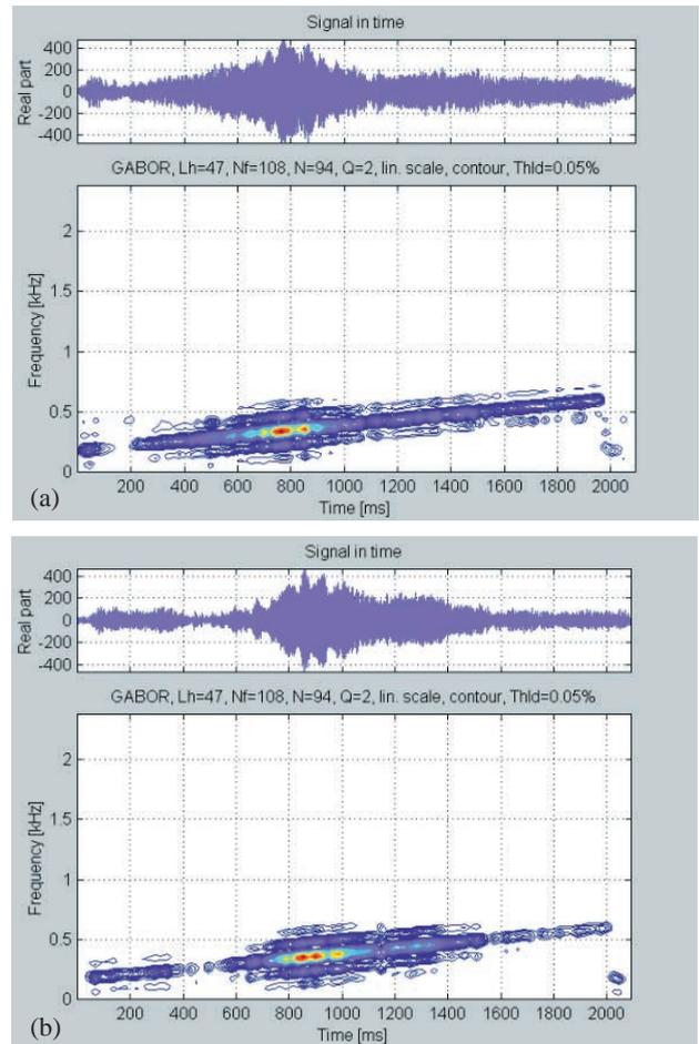
Figure 1. In both figures the beam signal over time (up) and the relative Gabor coefficients (down) are shown. (a) Signal acquired during low tide; (b) signal acquired during high tide.
