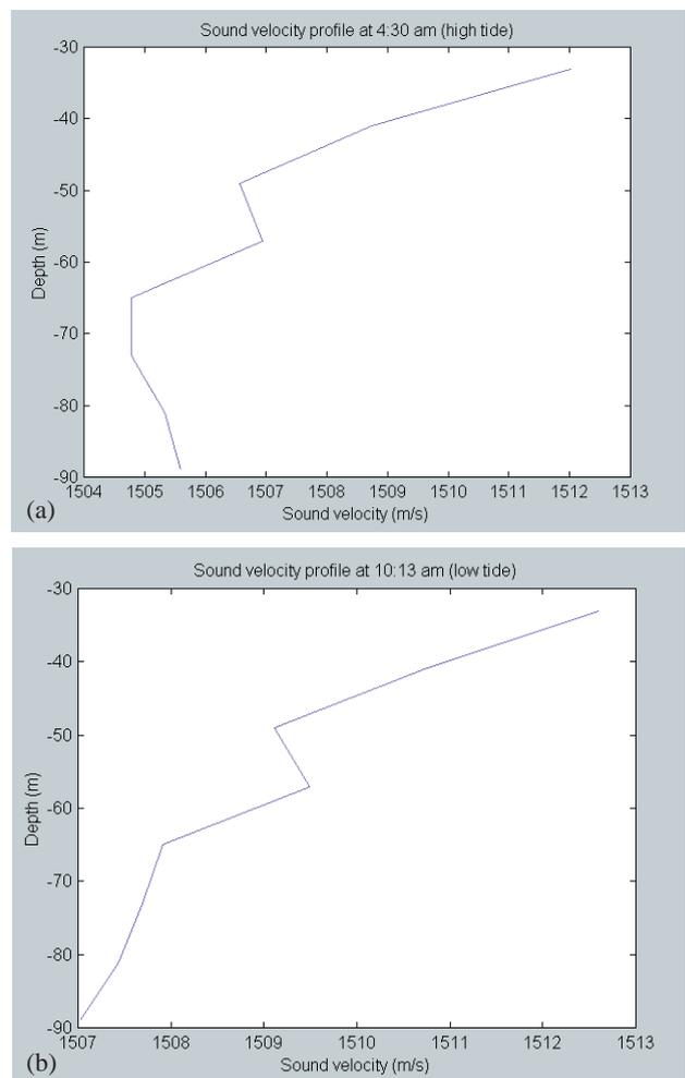
Figure 4. Sound velocity profile at two different hours of the day. (a) High tide period; (b) low tide period.
