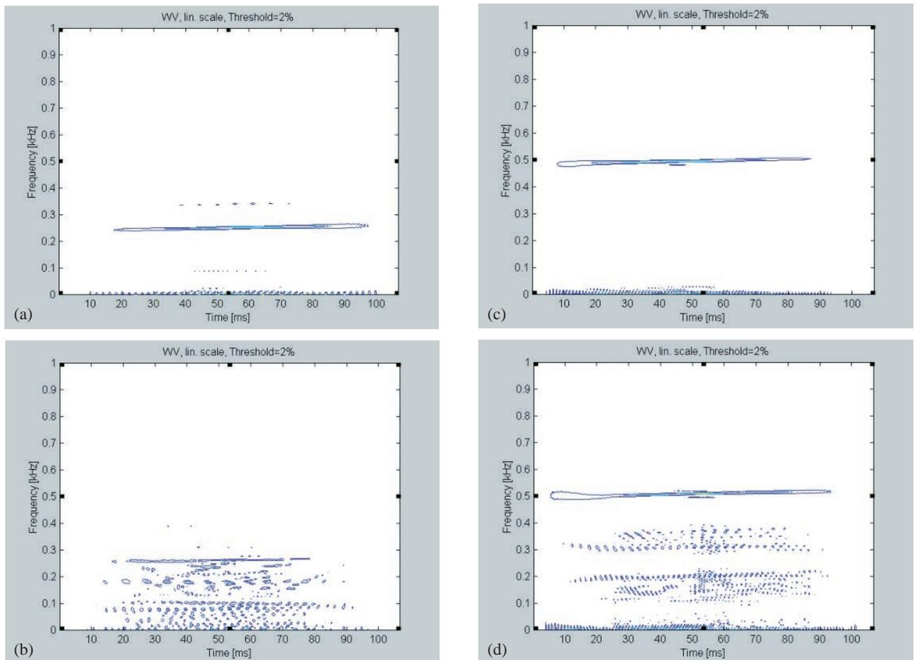
Figure 2. Wigner-Ville Distribution of specific signal portions. (a and c) Low tide and (b and d) high tide conditions.
