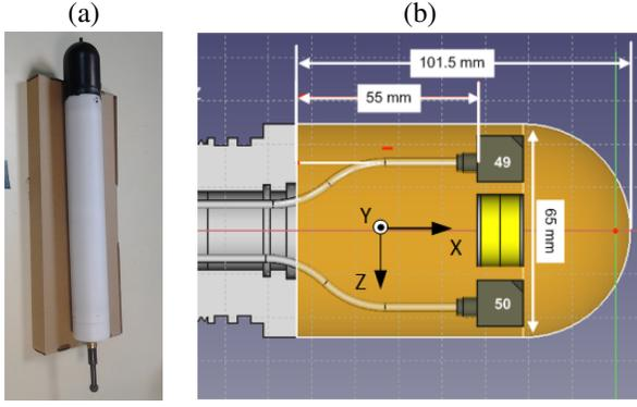
Fig. 1. Photo of the DAVS device: the black nose is the acoustic sensing part, the white Delrin container houses the electronics (including the batteries) (a). Acoustic sensing part (black nose) showing the position of the two tri-axial accelerometers (grey blocks, labeled as #49 and #50), the hydrophone (yellow cylinder) between them, and their position relative to the Cartesian coordinate system (b).
