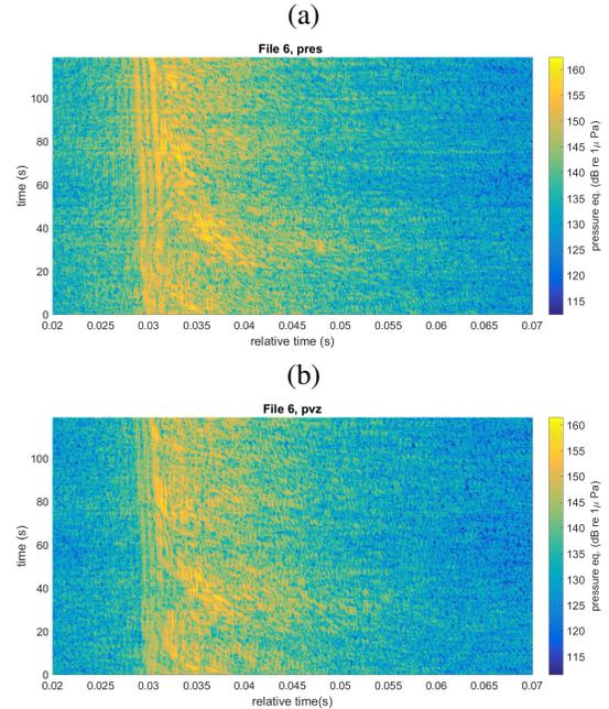
Fig. 7. Block of 120 s of pressure data (a) and combination of pressure and particle velocity acquired at 15:02 (b).
