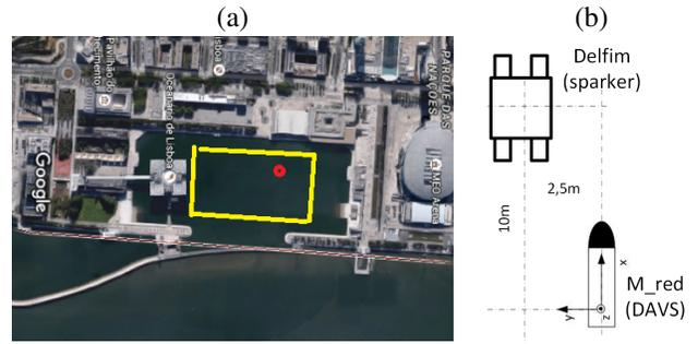
Fig. 3. The location of the experiment area delimited by the yellow line, inside of the Lisbon Oceanarium marina (a). Vehicle formation: the ASV Delfim carries the sparker and the red Medusa (M\_red) carries the DAVS (a).
