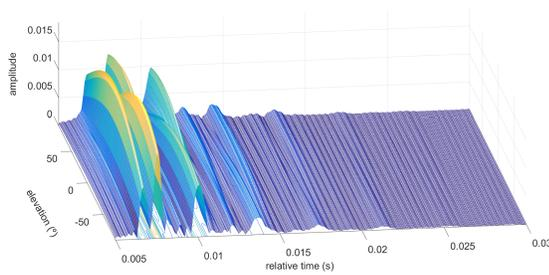
Fig. 2. Arrival patterns computed from signals generated by OASES, for the Oceanarium marina scenario (bottom parameters of Table I): pressure only (blue), combination of particle velocity and particle velocity gradient (red) and combination of pressure and particle velocity (black) (a), and combination of pressure and vertical and horizontal components of particle velocity steered for elevation angles between  $-90^\circ$  (bottom) and  $90^\circ$  (surface) (b).
