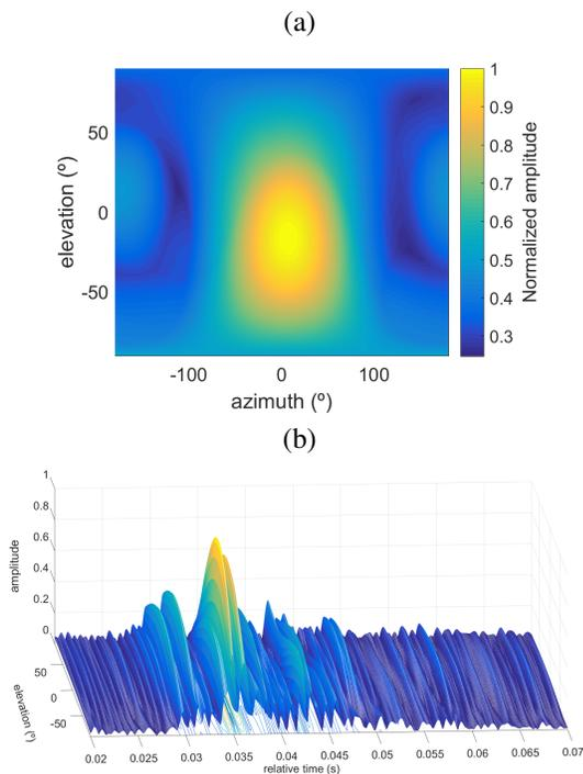
Fig. 8. Azimuth-elevation normalized ambiguity surface obtained for the highest peak in time domain (a) and corresponding 2D slice (elevation-time) for the azimuth fixed at the peak value (b), at second 39 from run start of the block of data shown in Fig. 7
