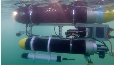
Fig. 4. The DAVS mounted beneath the MEDUSA AUV
