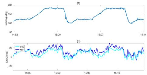
Fig. 6. Heading of the Medusa AUV measured by the DAVS motion sensor (a), azimuth of the sparker estimated from DAVS acoustic data using accelerometer #49 (cyan) an #50 (blue) (b).
