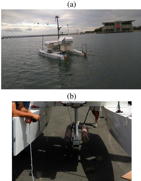
Fig. 5. The ASV Delfim (a). View of the sparker installed in the Delfim vehicle (b).
