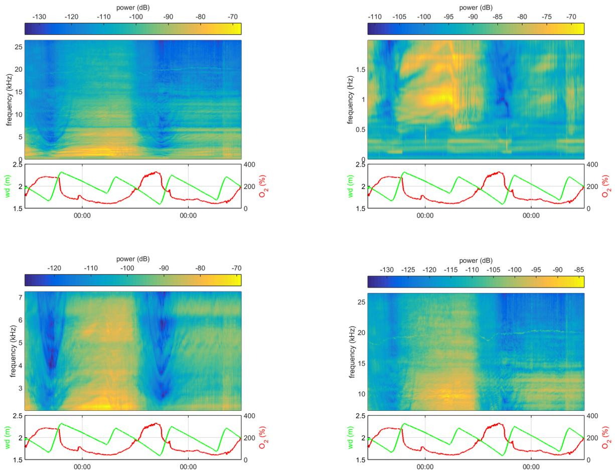
**Figure 3: Power spectral density of the ambient noise estimated every 10 min during 2 diurnal periods: full 0–25 kHz band (upper-left), and zoom of 0–2 kHz (upper-right), 2–7.25 kHz (bottom-left) and 7.25–25 kHz (bottom-right) bands. The red and green curves represent the O<sub>2</sub> saturation and water depth, respectively.**
