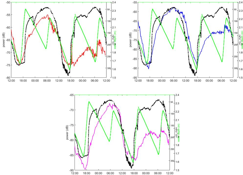
**Figure 4:** Comparison between the variability of the noise power in the bands 0–2 kHz (red), 2–7.25 kHz (blue) and 7.25–25 kHz (magenta), and the variability of O<sub>2</sub> saturation level (black). The green line represents the water depth (estimated from CTD).
