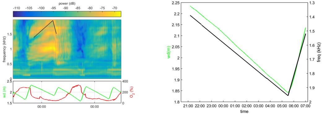
**Figure 5: Striation pattern due to water depth variability: spectrogram with superimposed striation curve (left), and comparison (right), where the black curve represents the striation and the green curve represents water depth.**
