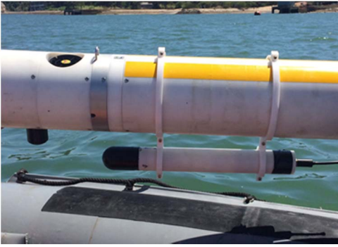
Figure 1 – A photo of the DAVS beneath the MARES before deployment
