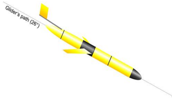
Figure 5 - Example of a slocum glider diving profile (source: Equipping an underwater glider with a new echosounder to explore ocean ecosystems , K. J. Benoit-Bird)
