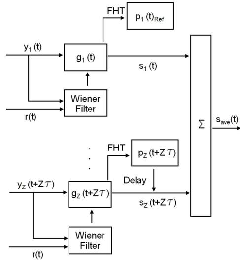
Fig. 3. Diagram of Wiener filtering, CIR estimation using Hadamard transform and coherent averaging of sequences whose TCOH was above the 0.6 threshold.
