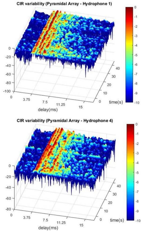
Fig. 2. CIR variability in time, estimated using 50 bitstreams ( $F_c$ :7.5 kHz,  $BW$ : 3 kHz). Data were recorded by hydrophone #1 (top plot) and #4 (bottom plot), installed at the top (1m above the bottom) and at the base of the pyramidal array.
