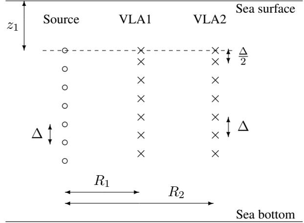
**Figure 1.** Illustration of source and sensor locations.
