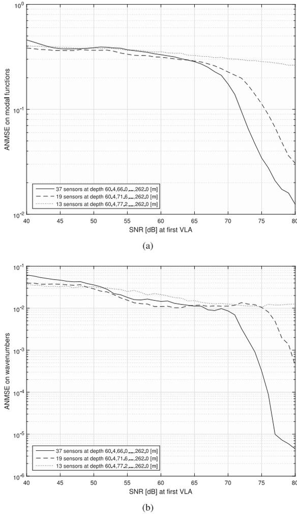
Fig. 7. Estimation accuracy for the 13-mode waveguide, as function of the observation SNR and the intersensor spacing, for two VLAs placed at 200 and 400 [m] from the source. The SNR at the second VLA is 3.8217 (resp., 3.7467 and 3.6655) [dB] lower than that at the first VLA, when sensors are spaced by 5.6 (resp., 11.2 and 16.8) [m].
