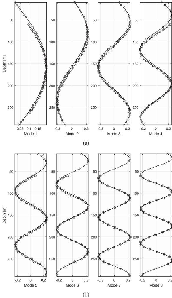
Fig. 5. Exact (“x”-dots) and estimated (“o”-dots, after amplitude and sign corrections) modal functions of the 8-mode waveguide. The two VLAs are placed at 200 [m] and 400 [m] from the source, with respective SNRs of 31.7384 and 27.9169 [dB], corresponding to  $\sigma_n = 10^{-4}$ .
