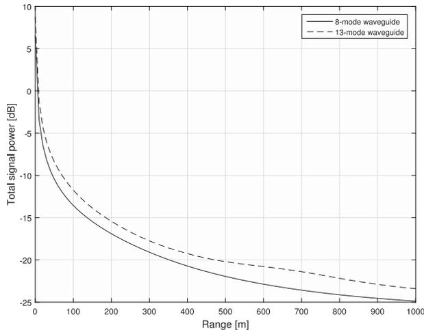
Fig. 3. Total signal power collected by a VLA as function of its range to the source. The 37 sensors are deployed at depths 60.4, 66, . . . , 262 [m].
