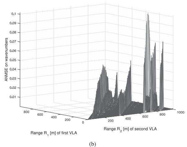
Fig. 4. Estimation accuracy as function of the range of the VLAs made, each, of 37 sensors deployed at depths 60.4, 66, . . . , 262 [m]. The 8-mode waveguide is corrupted by an AWGN characterized by a standard deviation  $\sigma_n = 10^{-4}$ .
