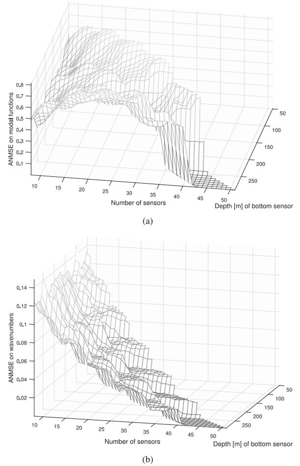
Fig. 8. Estimation accuracy for dense VLAs of all possible sizes and positions, deployed at 200 [m] and 400 [m] from the source. The 8-mode waveguide is corrupted by an AWGN characterized by a standard deviation  $\sigma_n = 10^{-4}$ .
