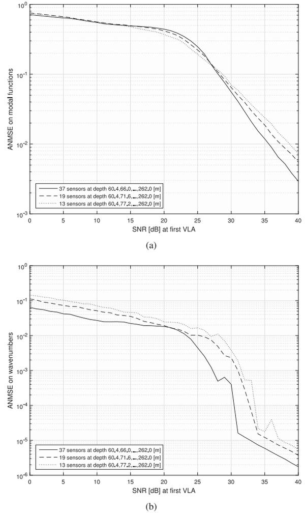
Fig. 6. Estimation accuracy for the 8-mode waveguide, as function of the observation SNR and the intersensor spacing, for two VLAs placed at 200 and 400 [m] from the source. The SNR at the second VLA is 3.8215 (resp., 3.7829 and 3.7435) [dB] lower than that at the first VLA, when sensors are spaced by 5.6 (resp., 11.2 and 16.8) [m].
