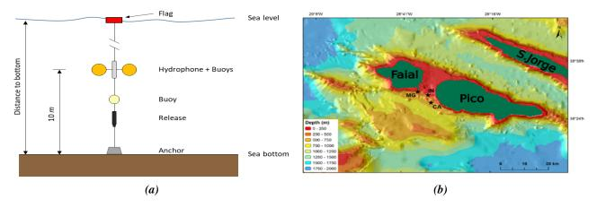
Figure 3: Experimental deployment setup: a) fixation system description and b) hydrophone location.
