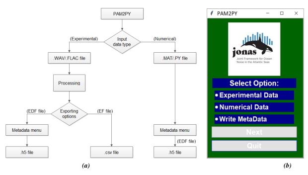
Figure 2: PAM2PY structure a) and interactive interface b).
