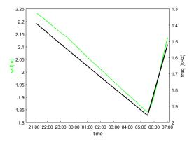
Figure 5: Striation pattern due to water depth variability: spectrogram with superimposed striation curve (left), and comparison (right), where the black curve represents the striation and the green curve represents water depth.
