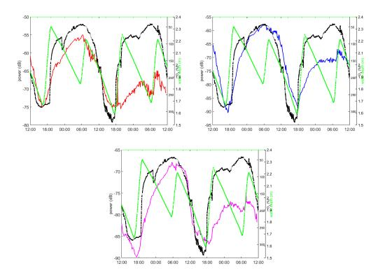
Figure 4: Comparison between the variability of the noise power in the bands 0–2 kHz (red), 2–7.25 kHz (blue) and 7.25–25 kHz (magenta), and the variability of O2 saturation level (black). The green line represents the water depth (estimated from CTD).
