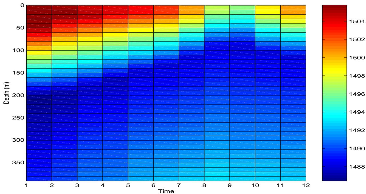
Figure 4.2: *Time variations of the sound-speed profiles in the middle cell. These profiles define the true environment.*
