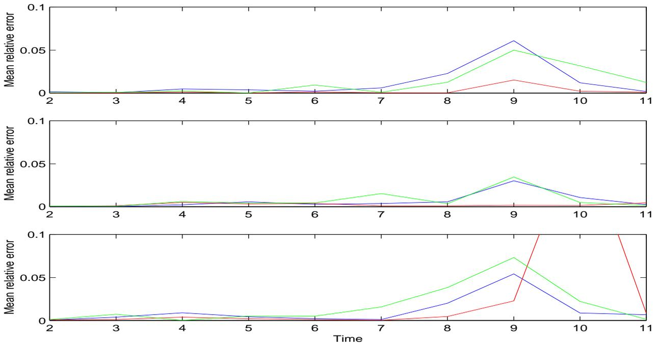
Figure 4.6: Variations of the parameter mean relative error ( $\varepsilon$ ) with the middle cell location (top:  $R_1=5$  km, middle:  $R_1=11$  km, bottom:  $R_1=17$  km) and width (blue: 12 km, red: 7 km, green: 2 km).
