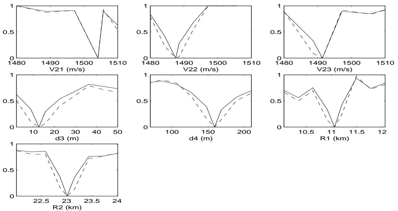
Figure 4.13: Variations of the misfit with individual parameter, the remaining parameters being fixed to their true value for time window 4, cell width 12 km and distance from source 11 km. The dash line indicates the noise-free case. The solid line shows the average misfit obtained for 15 realizations of correlated noise with SNR=5dB.
