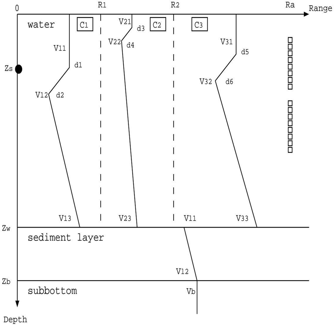
Figure 2.1: Model of the ocean waveguide. The acoustic source is located at range  $0$ , the vertical line of receivers at range  $R_a$ .
