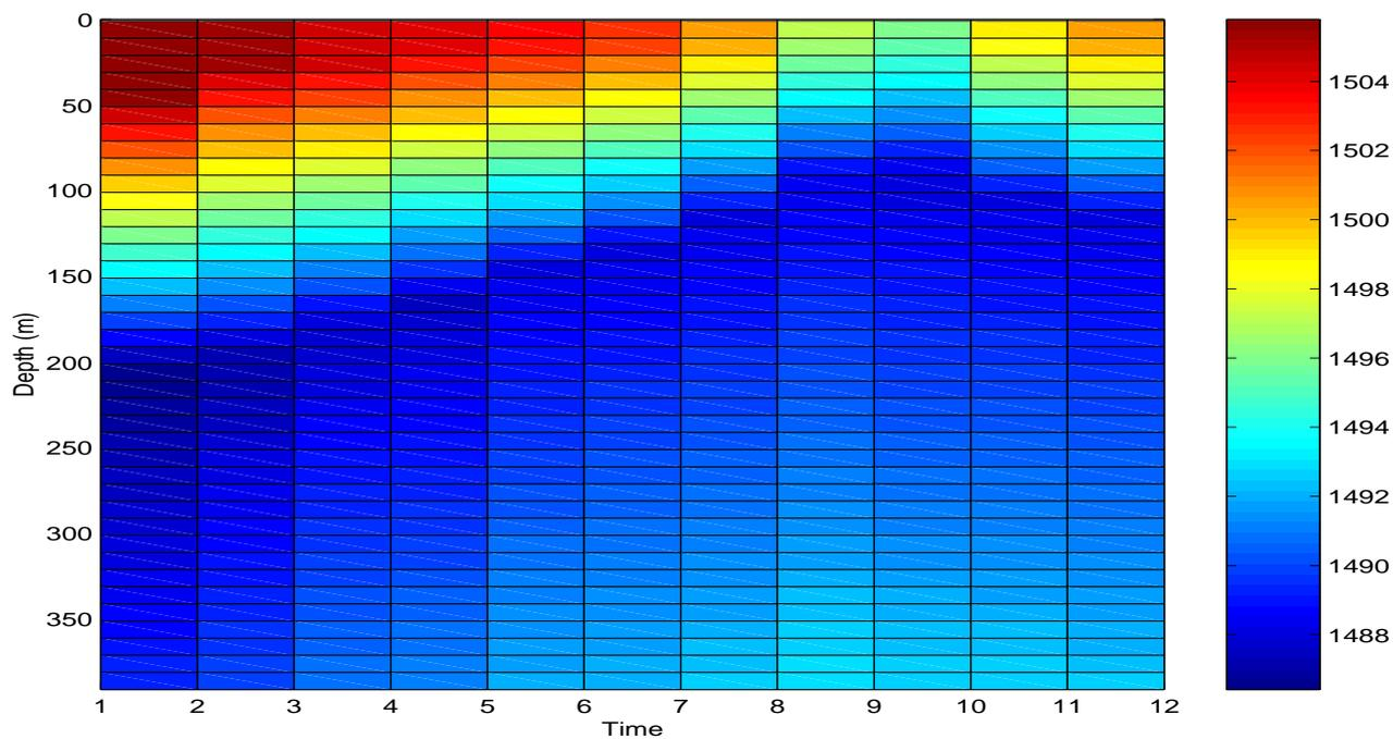
Figure 4.3: *Estimated sound-speed profiles in the middle cell.*
