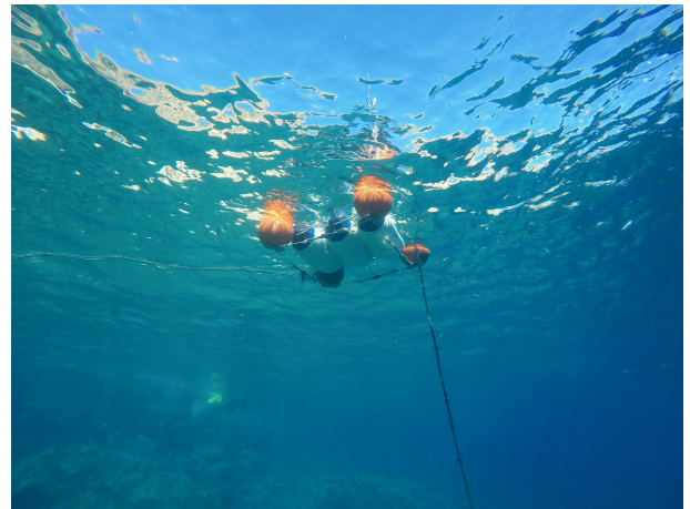
Figure 2.5: Equipment moored during the experiment. On the left the structure with the transducers placed above the marine plants; on the right the buoy with electronic devices and batteries floating near the anchored structure area.
