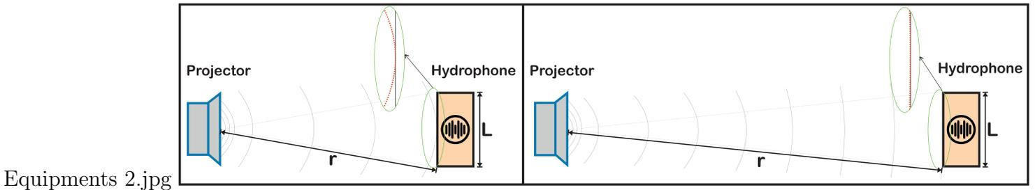
Figure 2.2: Free Field representation of a plane wave. Left side image shows a spherical wave in near field, where the wave curvature can be seen (dashed red line). Right side shows the receiver at a far field side showing that the wave is approximately plane.
