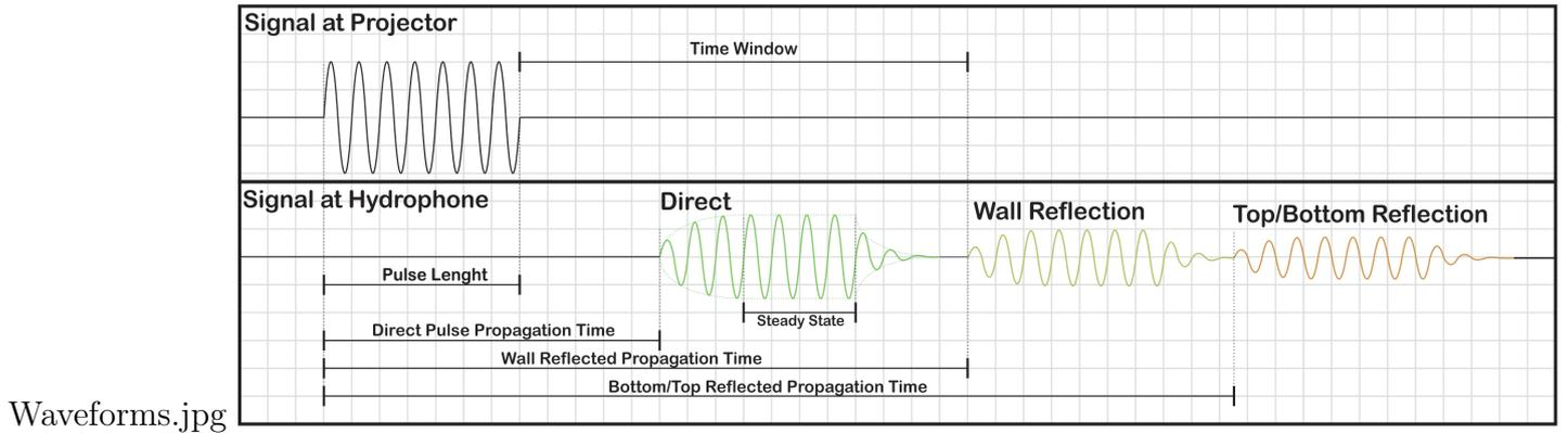
Figure 5.3: Underwater signals example for a tank experiment with pulsed signals. On top there's a single pulsed signal which last 7 cycles. On bottom, there are the three types of signals received, with the propagation times marked. The time window represent the free from reflections time and steady state the area of direct signal used for signal processing.
