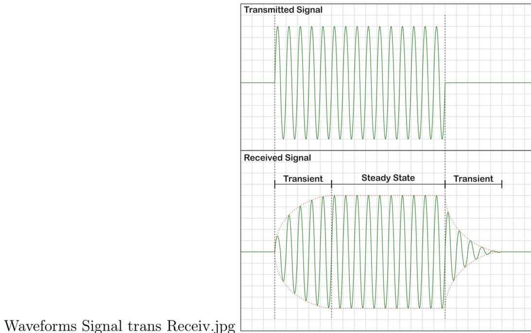
Figure 5.2: Example of a transmitted pulse (ideal) and received pulse without interferences, showing the transient and steady state parts of signal.
