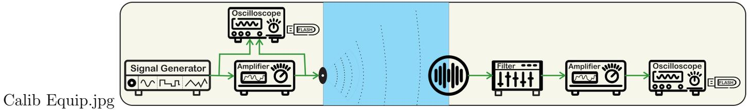
Figure 4.1: Common setup schematic for calibrating underwater acoustic transducers using comparison method. The blue part represents the water body.
