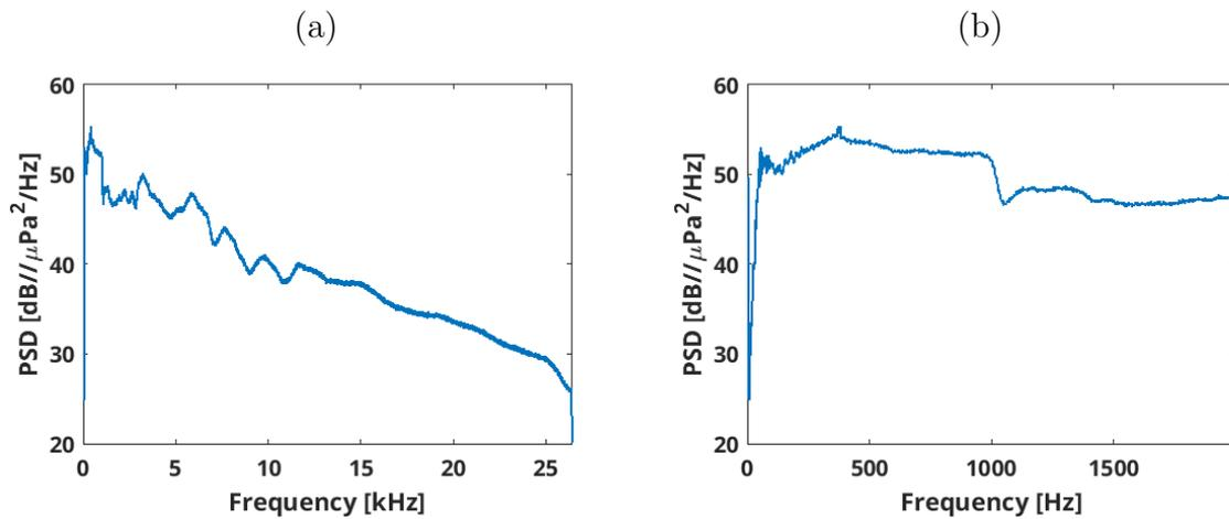
Figure 4.8: Mean spectral power density for the SR1B recorder data located in the channel (IN) mooring for the full 26 kHz band (a) and for the 2 kHz low band (b).
