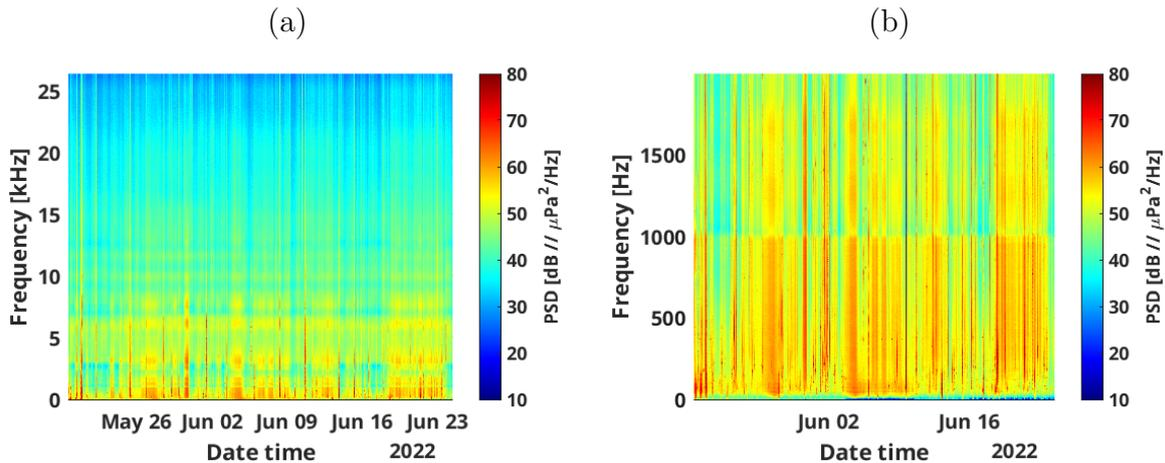
Figure 4.4: *Spectrogram for the SR1A recorder data located at Monte da Guia (MG) mooring for the full 26 kHz band (a) and for the 2 kHz low band (b).*
