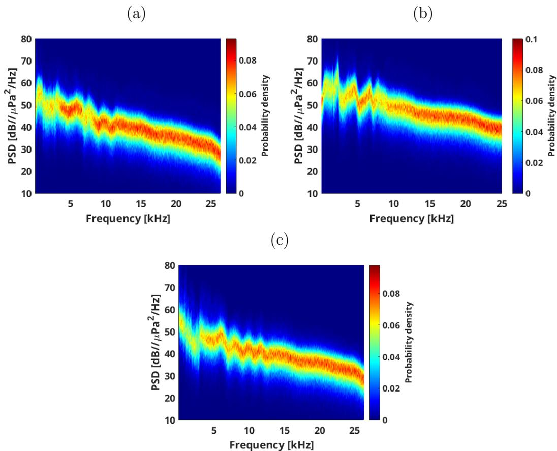
Figure 4.12: Spectral probability density for the full band and SR1B dataset : SR1B (a), EAR at IN (b) and SR1A (c). Note that SR1B and the EAR are in the same mooring, while SR1A is approximately 4.5 km away.
