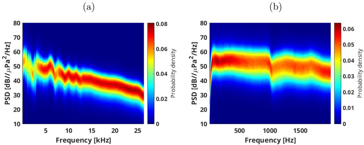
Figure 4.5: *Spectral probability density for the SR1A recorder data located at Monte da Guia (MG) mooring for the full 26 kHz band (a) and for the 2 kHz low band (b).*
