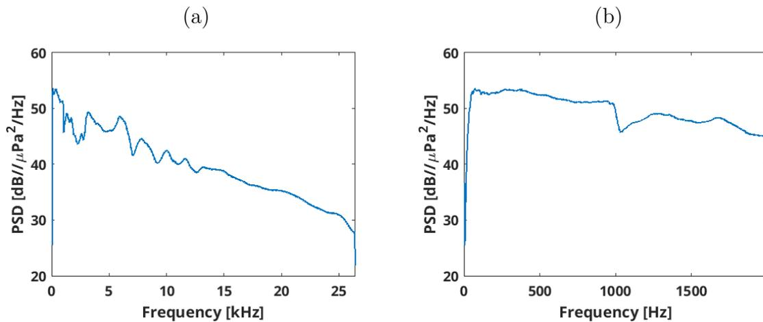
Figure 4.6: *Mean spectral power density for the SR1A recorder data located at Monte da Guia (MG) mooring for the full 26 kHz band (a) and for the 2 kHz low band (b).*
