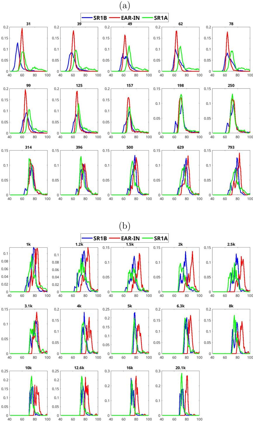
Figure 4.14: Histograms of the SPL data received at SR1B, EAR-IN and SR1A recorders for the 1/3 octave frequency bands for 20-1000 Hz (a) and 1-25 kHz (b).
