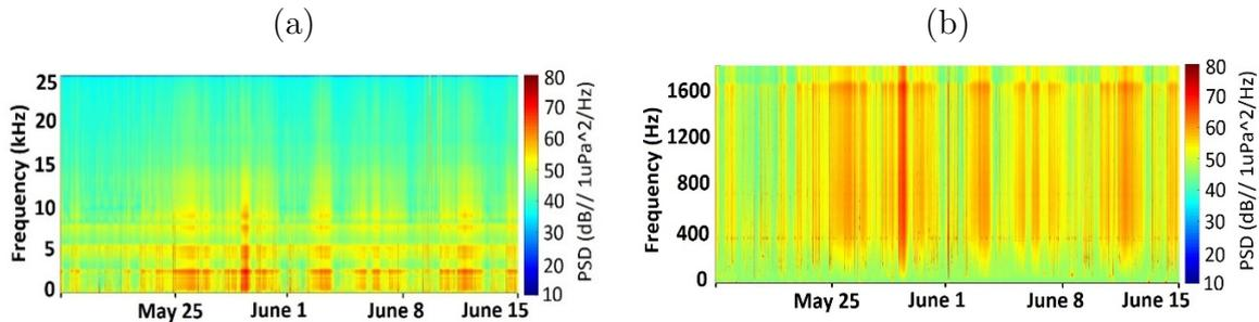
Figure 4.10: *Long term spectral average (LSTA) spectrogram at a resolution of 1 Hz for the full 25 kHz band (a) and for the low 2 kHz band (b) at IN location.*
