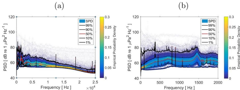
Figure 4.16: *Power spectral density (PSD) for the full 25 kHz band (a) and for the low 2 kHz band (b) at N location.*
