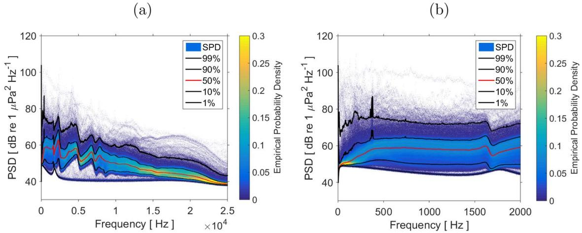
Figure 4.11: *Power spectral density (PSD) for the full 25 kHz band (a) and for the low 2 kHz band (b) at IN location.*
