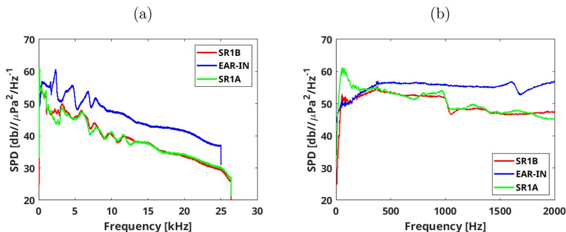
Figure 4.13: Mean spectral power density for the SR1B, EAR-IN and SR1A recorders data located in the channel (IN) mooring for the full 26 kHz band (a) and for the 2 kHz low band (b).
