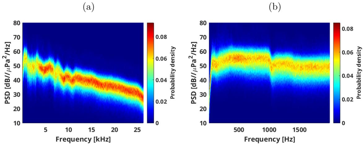
Figure 4.7: Spectral probability density for the SR1B recorder data located in the channel (IN) mooring for the full 26 kHz band (a) and for the 2 kHz low band (b).
