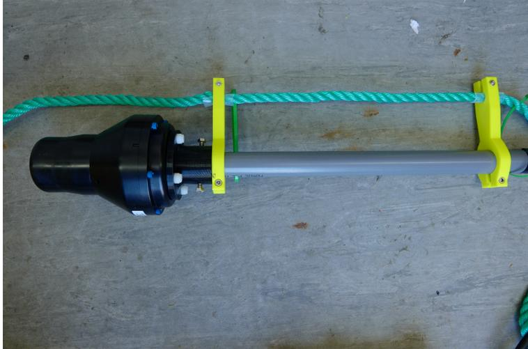
Figure 3.3: *M35 vector hydrophone support assembly for mooring.*
