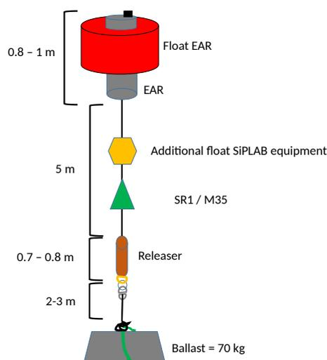
Figure 3.2: *Mooring design: two moorings with SR1 and one with M35 vector hydrophone.*
