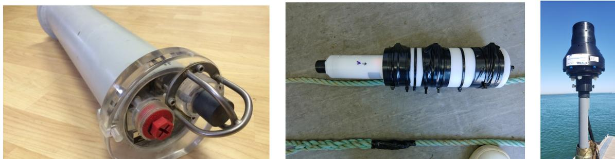
Figure 3.1: *Equipment: EAR (left), SR1 (middle) and Geospectrum M35 (right).*
