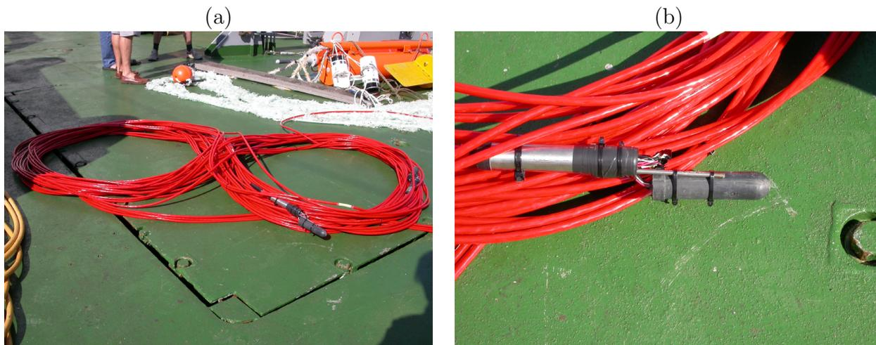
Figure 2.6: *Acoustic Oceanographic Buoy (AOB): hydrophone array (a) and pre-amplifier hydrophone package (b).*
