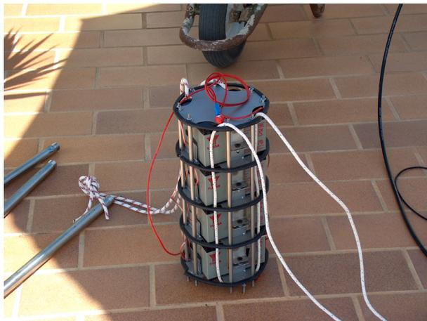
Figure 2.5: *Acoustic Oceanographic Buoy battery pack.*
