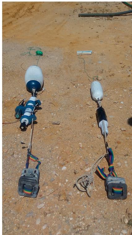
Figure 2.2: The CTD (left mooring) and SR-1 (right mooring) moorings before deployment.
