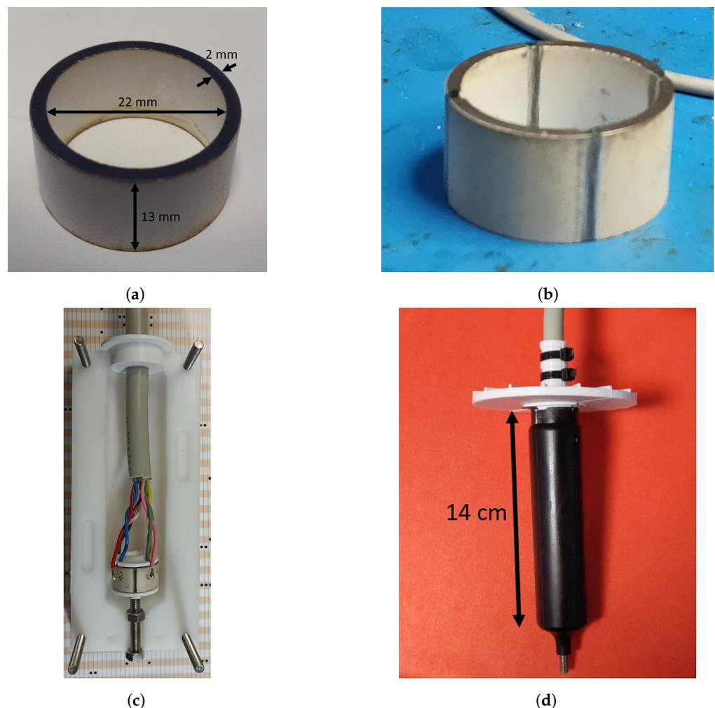
**Figure 3.** Prototype manufacturing: (a) piezoceramic hollow cylinder made of PZT-4; (b) piezoceramic cylinder, with eight aligned rips; (c) prototype of the spiral source in the potting frame, before the polyurethane potting; (d) prototype of the spiral source after the polyurethane potting, with a bearing angle reference frame on the top.
