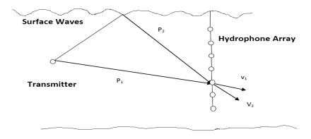
Figure 2.Two arrivals from transmitter to the receiver and their velocity projections
