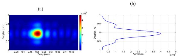
Figure 7. (a) Doppler computed only for 4 sec time window where we can see three Dopplers i) due to one main arrival at 0.1 Hz and ii) due to a top reflected arrival at ~-0.4 Hz and at ~0.5 Hz, (b) Doppler summation over the delay axis
