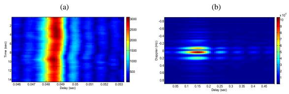
Figure 5. Doppler Spectrum for the selected arrival for 15 seconds
