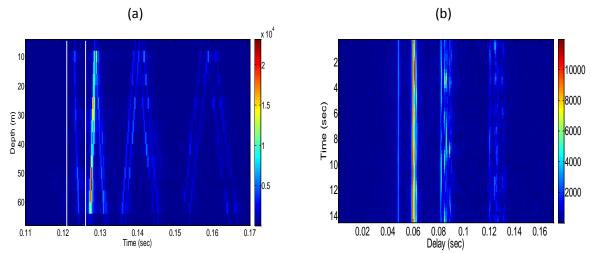
Figure 4: Impulse response estimates: (a) for 16 Hydrophone array and white lines showing the selected arrival; (b) for channel 3 along the 15 seconds
