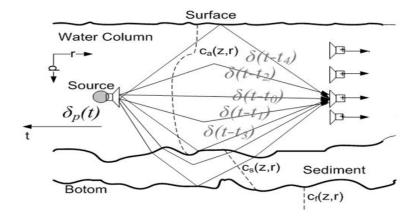
Figure 1. Underwater Environment with source transmitting impulses which reach the hydrophone array through different paths
