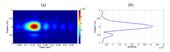
Figure 6. (a) Doppler computed only for 4 sec time window where we can see two Dopplers i) due to one main arrival at -0.01Hz and ii) due to a surface reflected arrival at approximately 0.5 Hz (b) Doppler summation over the delay axis
