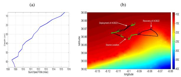
Figure 3: (a) Down reflecting sound speed profile during Day 2; (b) Day 2 bathymetry map of the work area with GPS estimated locations of AOB21 (A1d) and AOB22 (A2d) deployments and their recovery (A1r,A2r), ship/source track (dotted line) and ship track during field calibration events (green lines).
