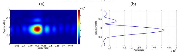
Figure 8. (a) Doppler computed only for 4 sec time window where we can see two Dopplers i) due to one main arrival at 0.1 Hz and ii) due to a top reflected arrival at  $\sim$  -0.4 Hz, (b) Doppler summation over the delay axis
